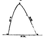
When this plate has been curved on the model, it fits the body of the plough very well, and carries the furrow slice on to the mould-board with the least possible degree of friction.
